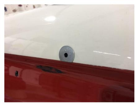
Use 10-24 fender washer a (McMaster 91525A115) on the inside of the fender. Trim the washers to fit the curvature of the fender and door for the top moldings - (grind about 30% off one side of the washer). The 10-24 nuts are **McMaster** 96278A011, nut with external tooth lock washer built on it (in picture above).
