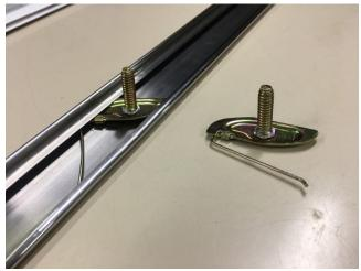
Top molding: rear clip (next to door) - must use this clip because you have no access to install a nut). One Napa 665-2864 plastic push clip. Make a spacer out of stainless (.035") with a 11/32<sup>nd</sup> inch hole centered, to shim the springloaded part of the clip. Make the spacer fit the curvature of the stainless trim.
