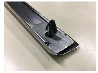
Lower molding: the front 6 clips are Napa 665-1141 – metal spring tee clip. Remove fresh air tube from inside the car to gain access to the rear clip.
