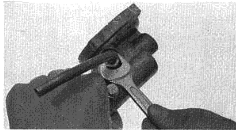
Fig. 11A-19 Vacuum Pipe Removal
