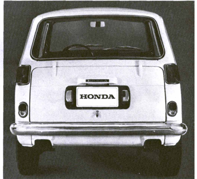
With skimpy bumper, protection at the rear of the Honda is minimal. Overrides appear a necessity. Well planned location of the taillights will assure that the small car will be seen.
