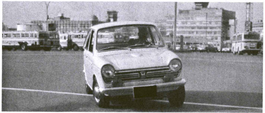
Front wheel drive makes the Honda 600 a cornering little demon. While a rear wheel will lift in a tight turn there is no loss of adhesion with the driving wheels pulling.
